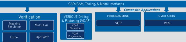
**VERICUT's modular format provides flexibility** - purchase only the capabilities you need. It's easy to add modules; just contact us and we will provide a license that gives you immediate access. VERICUT runs on Windows platforms as a 64 bit application. G-codes and CAM center-line (CL) formats are supported.
