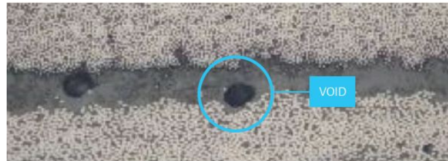
Structure contains voids
