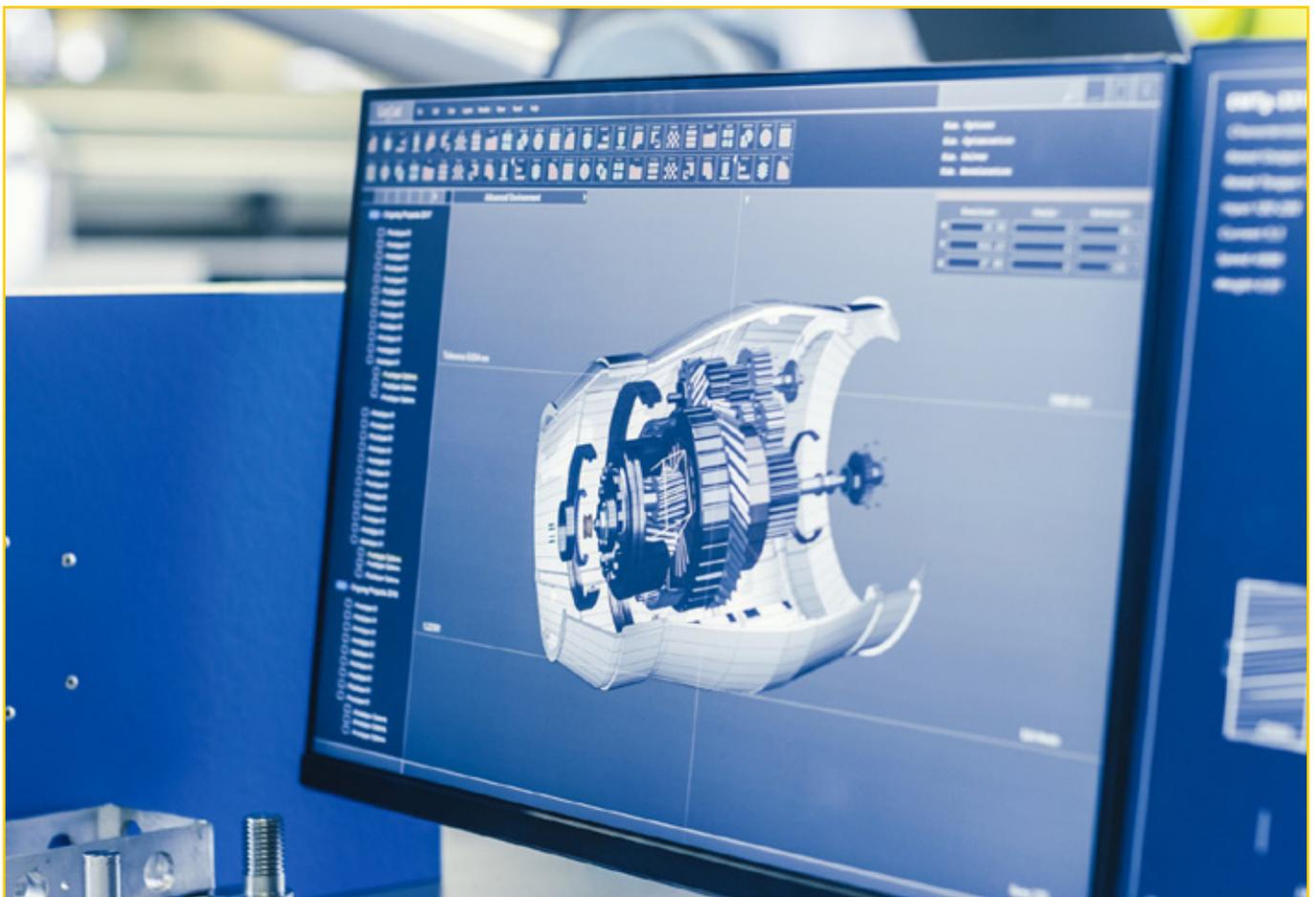
A digital twin digitally replicates a physical asset in the virtual environment.
