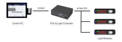
Each light module is assigned a unique address via the issue of an address assignment command whilst the confirm button on the target module is being held. This quick and simple mechanism allows for **rapid reconfiguration** and/or module swap-out should there be the need.
