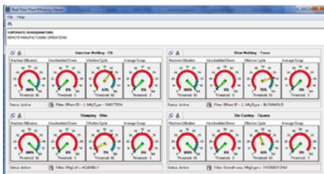
Overall efficiency views - with drill down to individual work centers - shows overall machine utilization, unscheduled downtime, effective cycle time and average scrap for each work cell or business unit.
