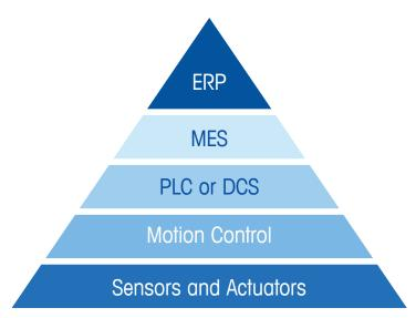
Traditional ISA95 SCADA -Pyramid illustrating the hierarchy in Automation.
