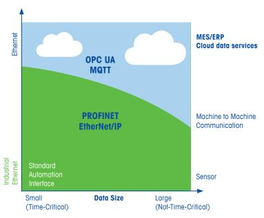
Illustration of application ranges of different communication technologies.
