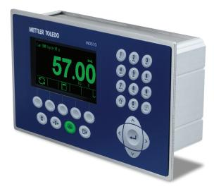
IND570 Weighing terminal with HMI interface.
