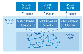
An OPC UA server is able to provide data for a multitude of clients inside and outside of the facility.
