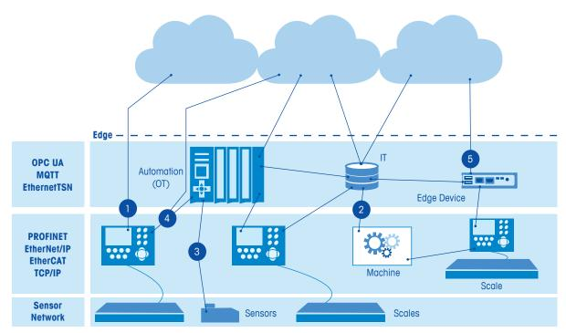
Overview of connectivity solutions for standalone and machine-integrated weighing devices.
